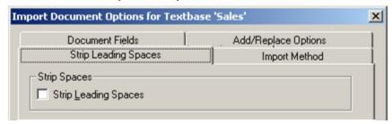
Check **Strip Leading Spaces** if you want to remove leading spaces during import. Clear the box if you want to retain leading spaces, which may have been included for formatting purposes, such as indentation. **Note**: Upon import, every tab (at the beginning of a line or embedded in the text) is converted to one space. This is true regardless of whether you check or clear this box.
