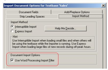
To extract text from binary (non-text) files, such as Microsoft Word documents or PDF files, IFilters must be installed on the Importer machine. Many IFilters are installed as part of the Windows operating system, but some may need to be installed manually. Please see *IFilters* in the Glossary. If IFilters are detected by the Importer, **Use Word Processing Import Filter** is checked by default.
